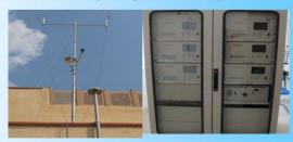
Presently, School of Earth Sciences had installed Ambient Air Quality Monitoring Station (AAQMS) for real-time data monitoring of common air pollutants including Ozone (O<sub>3</sub>), Nitrogen Oxides (NO<sub>2</sub>, NO, NOx), Carbon monoxide (CO), Sulphur dioxide (SO<sub>2</sub>), Methane (CH<sub>4</sub>) and Non-methane hydrocarbons (NMHC), and various meteorological parameters i.e., Rainfall, Temperature, Radiation, Humidity, pressure, Wind speed and direction.
